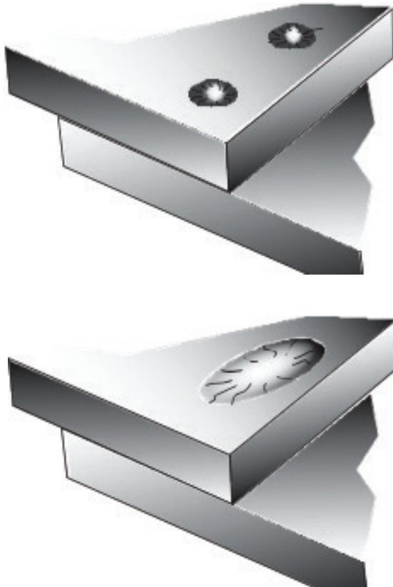
Plug Welds (Fig 1-19j)
